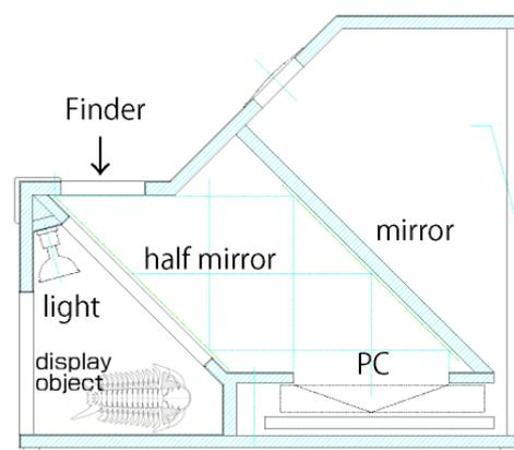
Fig. 3 Display box structure
