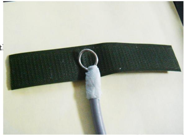
Fig. 2: Ring-shaped antenna
